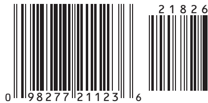
UPC A + Five-digit Supplemental (encoding 09827721123, supplemental = 21826)
