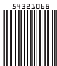
Interleaved 2-of-5 (encoding 54321068)
