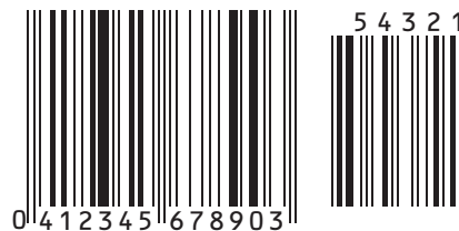
EAN + 5 Digit Supplemental (encoding 041234567890, supplemental = 54321)
