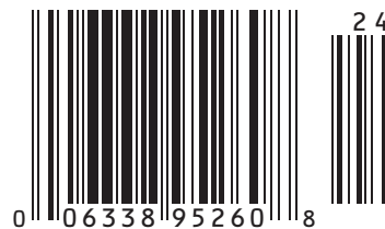
UPC A + Two-digit Supplemental (encoding 00633895260, supplemental = 24)
