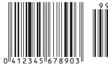
EAN + 2 Digit Supplemental (encoding 041234567890, supplemental = 99)
